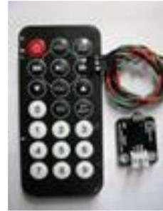
Gambar 2. *Transmitter dan Receiver Remote Control*
