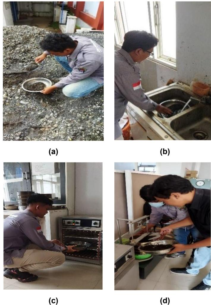
**Figure 6.** Sieve Gradation Testing Process
