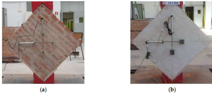
Figure 2. Set Up of Diagonal Shear Test Objects (Torres et al., 2020)
