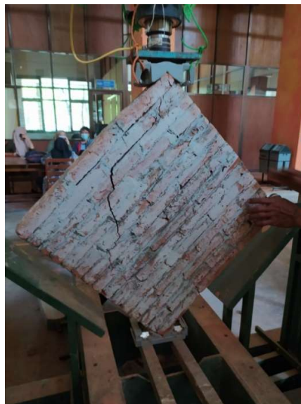
Figure 5. The laboratory specimen after the shear test
